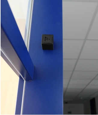
Fig. 7. KETCube as an RHT sensor fasten to a ferromagnetic surface
