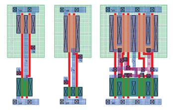
Fig. 2. Layout of NAND2X1 (4 x 10.8  $\mu$ m), NOR2X1 (4 x 10.8  $\mu$ m) and XOR2X1 (7.2 x 10.8  $\mu$ m) cells in 180nm TSMC technology
