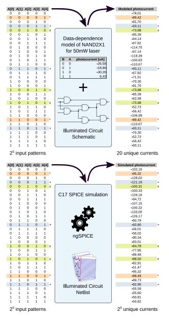
Fig. 14. Example of the data dependent power modeling for the C17 circuit; the C17 circuit is composed of 6 NAND2X1 standard cells; the *Modeled photocurrent* column shows the resulting currents for the composition of gate models and the *Simulated photocurrent* column shows the currents coming from the C17 netlist simulation
