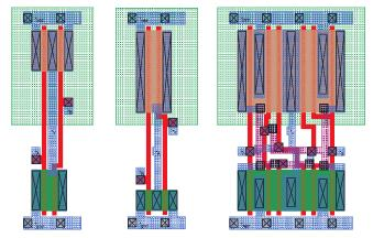
Layout of NAND2X1 (4  $\times$  10.8  $\mu m),$  NOR2X1 (4  $\times$  10.8  $\mu m)$  and XOR2X1 (7.2  $\times$  10.8  $\mu m)$  cells in 180nm TSMC technology
